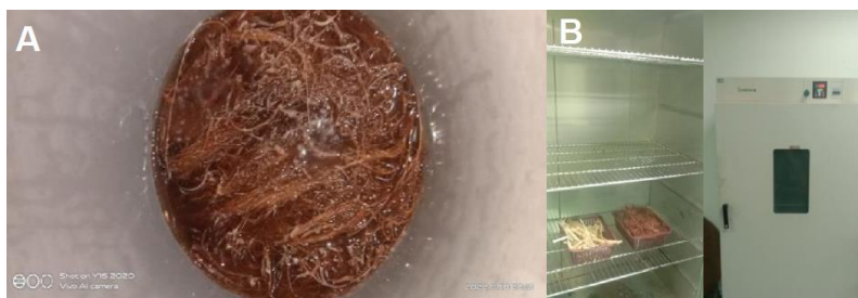
Figure 1 Natural fiber treatment; 1a) NaOH immersing and 1b) dried process
